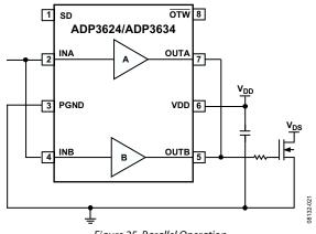
Figure 25. Parallel Operation
