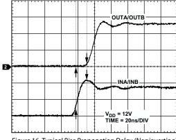
Figure 16. Typical Rise Propagation Delay (Noninverting)
