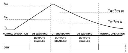
Figure 6. Overtemperature Warning and Shutdown
