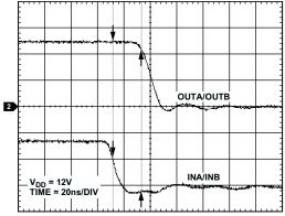
Figure 17. Typical Fall Propagation Delay (Noninverting)
