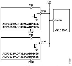
Figure 23. OTW Signaling Scheme Example
