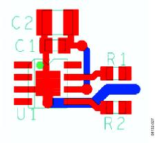
Figure 24. External Component Placement Example
