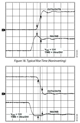
Figure 19. Typical Fall Time (Noninverting)
